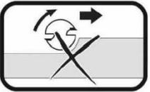
If the direction of travel is reversed, it may cause loss of control of the cutter
