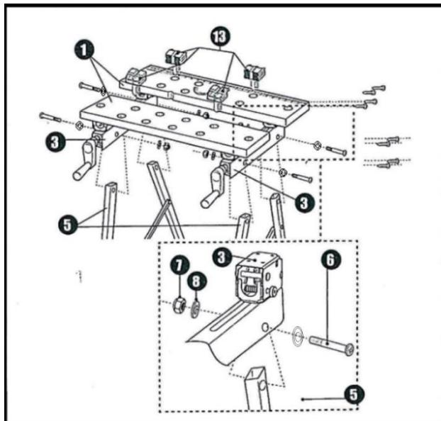
7. Insert support wedges (13) into the appropriate holes on the worktop work surface (1), depending on the dimensions of the workpiece to be machined
