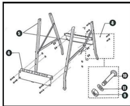
4. Install the crossbars (4) as shown in the picture and secure them to the legs (8) using bolts (10), washers (11) and nuts (9).
